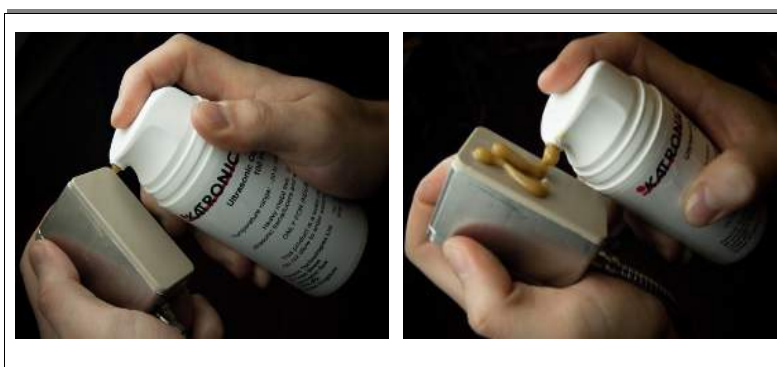
Illustration 5: Application of acoustic coupling gel
