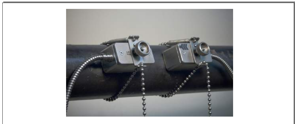
Illustration 7: Sensor mounting with clips and chains
