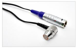
Wall thickness gauge NT with ODU/LEMO connector
