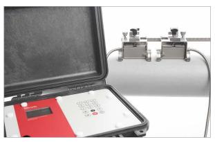
KATflow 210 with mounting rail and transducers
