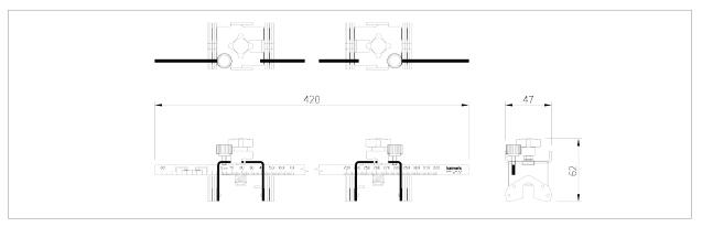
Mounting fixture, rail and magnets
