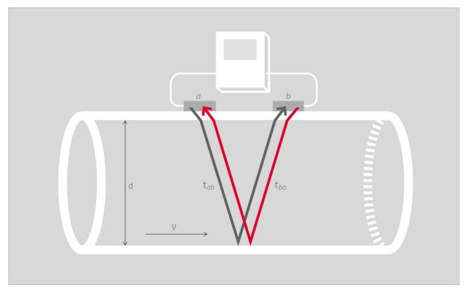
Sensors *a* and *b* work alternately to send and receive ultrasonic pulses. The sound waves *ab* travelling with the flow move faster than those travelling against it *ba*.
