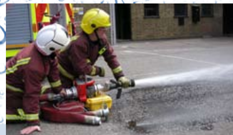
Using the Flowmaster to test fire fighting equipment
