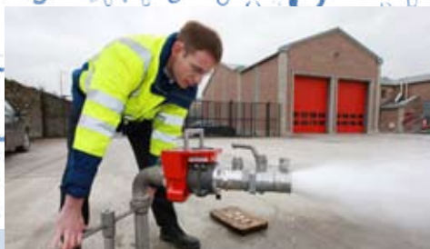
Measuring the static and dynamic pressure and the flow rate.
