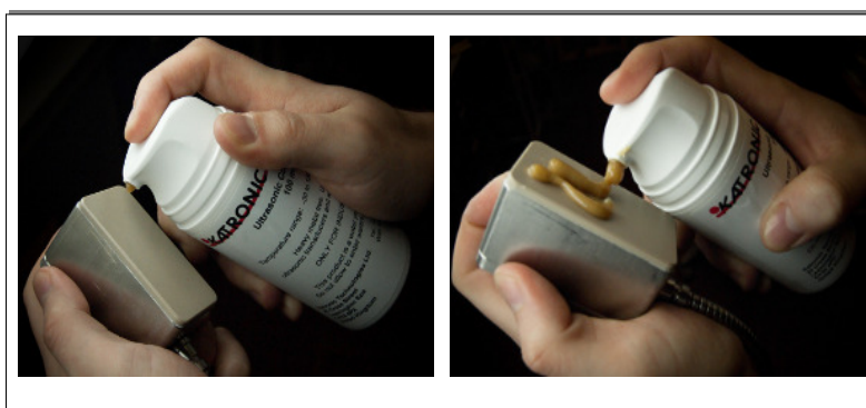
Illustration 7: Application of acoustic coupling gel
