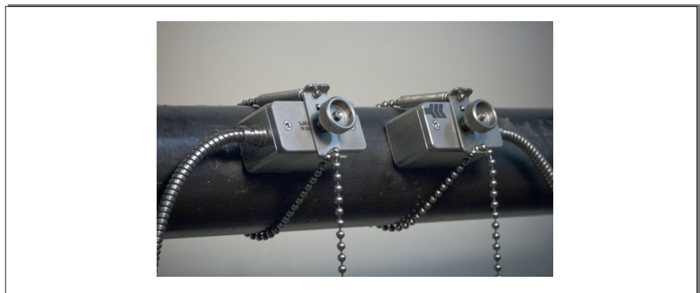
Illustration 9: Sensor mounting with clips and chains
