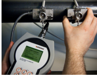
Illustration 6: Correct positioning of the sensors
