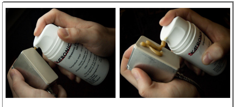
Illustration 5: Application of acoustic coupling gel
