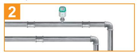
For stationary use there are the following outputs available for the data transfer to a building management system or PLC: 4...20 mA for actual consumption. Pulse output (galvanically separated) for the total consumption.
