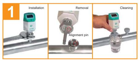
In most cases the compressed air in not free from oil, condensate, dirt and particles. In the course of time this leads to a soiling of the compressed air counters which may
