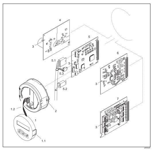
Fig. 34: Field housing: removing and installing printed circuit boards
