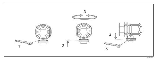
Fig. 14: Turning the transmitter housing (stainless steel field housing)
