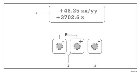
Fig. 26: Display and operating elements
