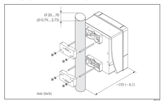
Fig. 17: Pipe mounting (wall-mount housing)
