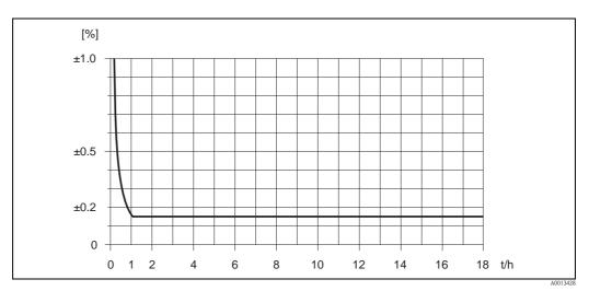
Fig. 42: Max. measured error in % o.r. (example: Promass P, DN 25)
