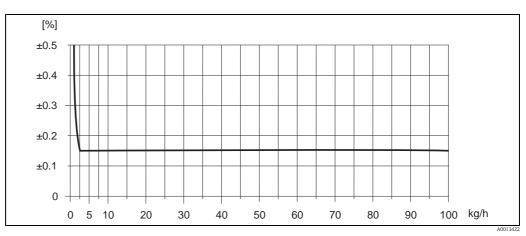
Fig. 37: Max. measured error in % o.r. (example: Promass A, DN 2)
