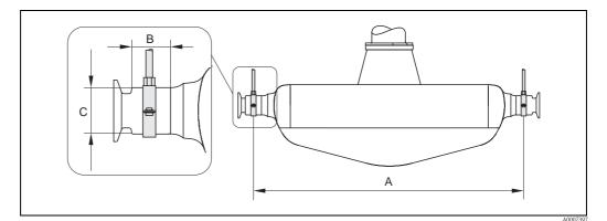
*Fig. 10: Promass P, mounted with mounting clamp*
