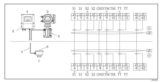
Fig. 19: Connecting the remote version
