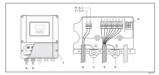
*Fig. 22:* Connecting the transmitter (wall-mount housing); cable cross-section: max. 2.5 mm<sup>2</sup>
