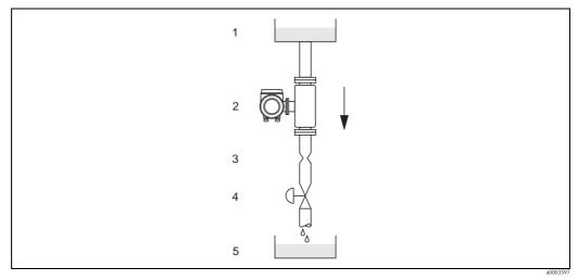
Fig. 6: Installation in a vertical pipe (e.g. for batching applications)
