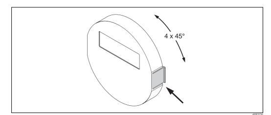
Fig. 18: Turning the local display (field housing)
