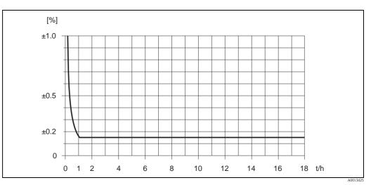
Fig. 40: Max. measured error in % o.r. (example: Promass H, DN 25)
