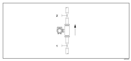
Fig. 32: Zero point adjustment and shutoff valves
