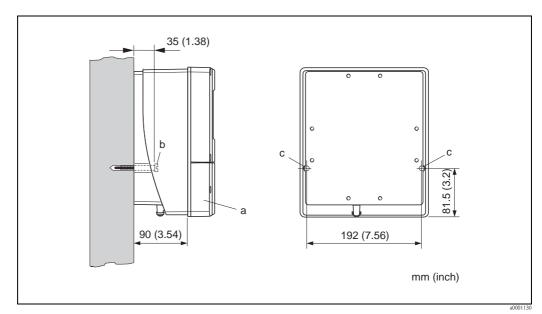
Fig. 15: Mounted directly on the wall
