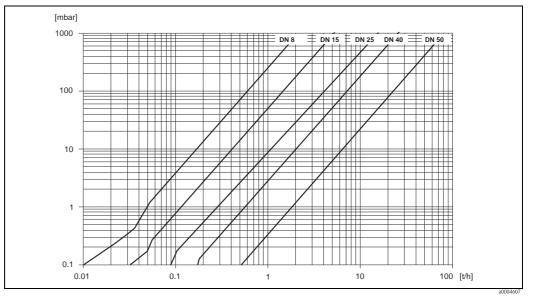
Abb. 49: Pressure loss diagram for water
