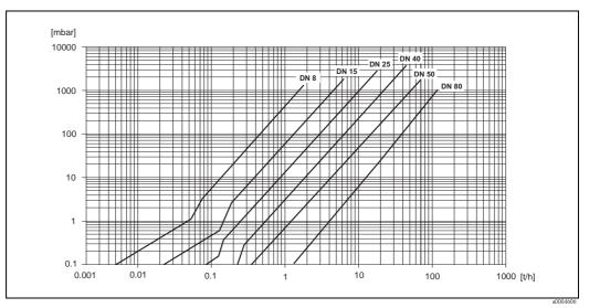
Fig. 45: Pressure loss diagram for water
