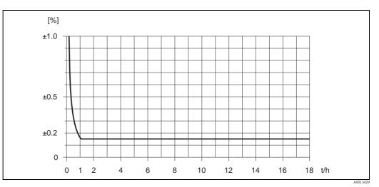
Fig. 43: Max. measured error in % o.r. (example: Promass S, DN 25)
