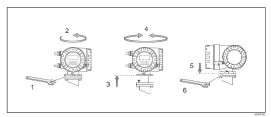
Fig. 13: Turning the transmitter housing (aluminum field housing)
