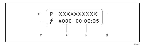
Fig. 28: Error messages on the display (example)
