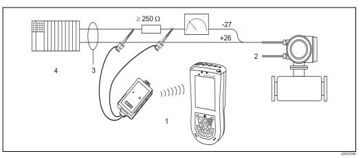
Fig. 23: Electrical connection of HART handheld terminal
