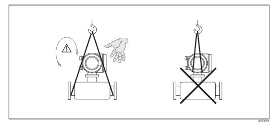
*Fig. 4:* Instructions for transporting sensors with > DN 40 (1 1/2")
