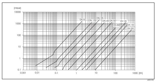
Fig. 44: Pressure loss diagram for water
