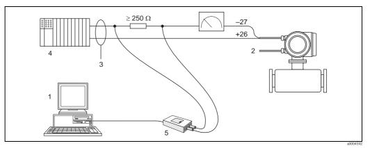
*Fig. 24: Electrical connection of a PC with operating software*
