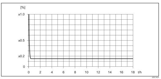
Fig. 39: Max. measured error in % o.r. (example: Promass F, DN 25)
