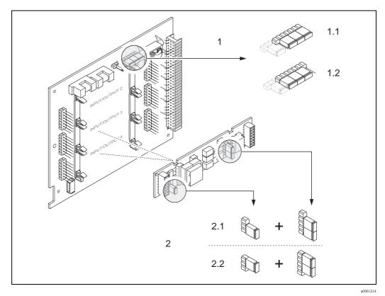
Fig. 31: Configuring current outputs with the aid of jumpers (I/O board)
