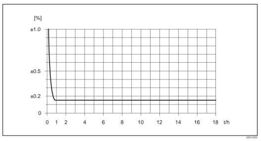
Abb. 41: Max. measured error in % o.r. (example: Promass I, DN 25)
