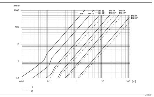
Fig. 48: Pressure loss diagram for water
