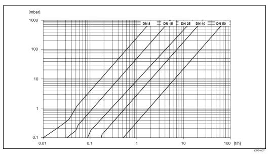
Fig. 47: Pressure loss diagram for water
