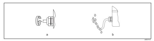
Fig. 25: Installation instructions, cable entries
