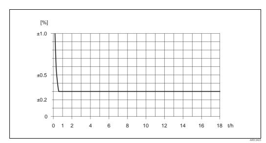
Fig. 38: Max. measured error in % o.r. (example: Promass E, DN 25)
