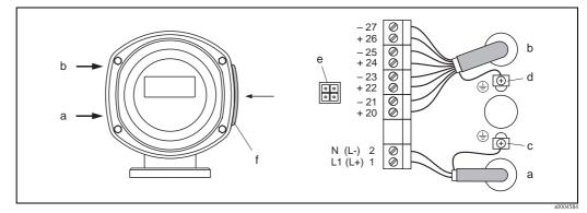
*Fig. 21:* Connecting the transmitter (stainless steel field housing); cable cross-section: max. 2.5 mm<sup>2</sup>
