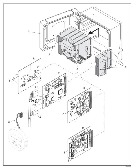
Fig. 35: Field housing: removing and installing printed circuit boards
