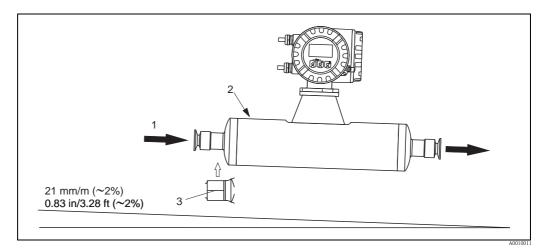
*Fig. 9:* Promass *I:* When lines are pitched in a specific direction and at a specific slope: as per hygienic guidelines (21 mm/m or approximatley 2%). Gravity can be used to achieve complete drainability.
