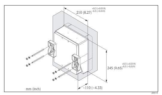
Fig. 16: Panel installation (wall-mount housing)
