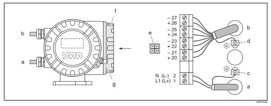
Fig. 20: Connecting the transmitter (aluminum field housing); cable cross-section: max. 2.5 mm<sup>2</sup>
