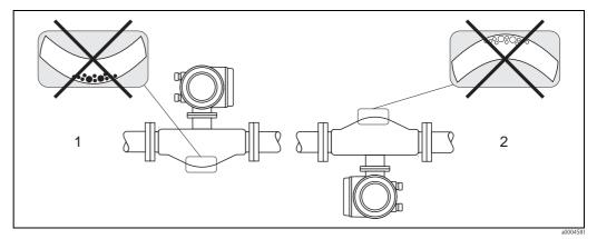
Fig. 7: Horizontal installation of sensors with curved measuring tube.
